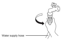
When dismantling, after turn off water tap, press start button and run for 10 seconds for prevent water from spilling out during dismantling then dismantle the water supply hose.
